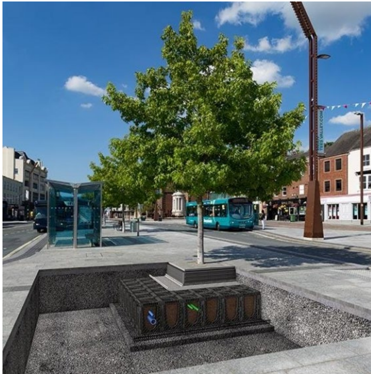
Graphic: GreenBlue Urban's RootSpace soil-cell system providing structured soil volume and utility space beneath paving in a street tree application.
