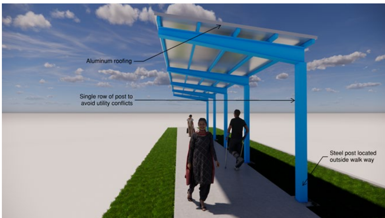
FIGURE 4-2. COVERED WALKWAY DESIGN USING ROOF WITH HIGH SOLAR REFLECTIVE INDEX AND HIGH ENOUGH ELEVATION TO REDUCE HEAT TRANSMISSION TO OCCUPANTS
