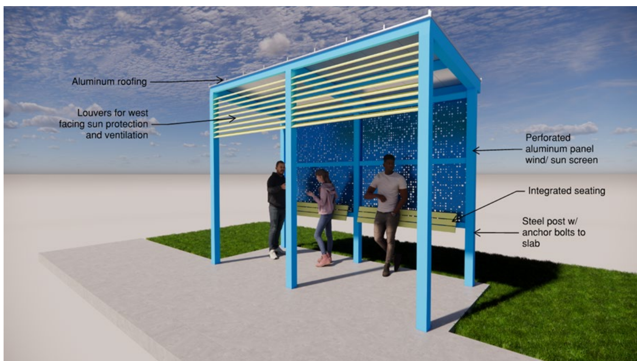
FIGURE 4-4. BUS SHELTER DESIGN USES PERFORATED PANELS AND LOUVERS TO MAXIMIZE SUN SCREENING AND ALLOW VENTILATION
