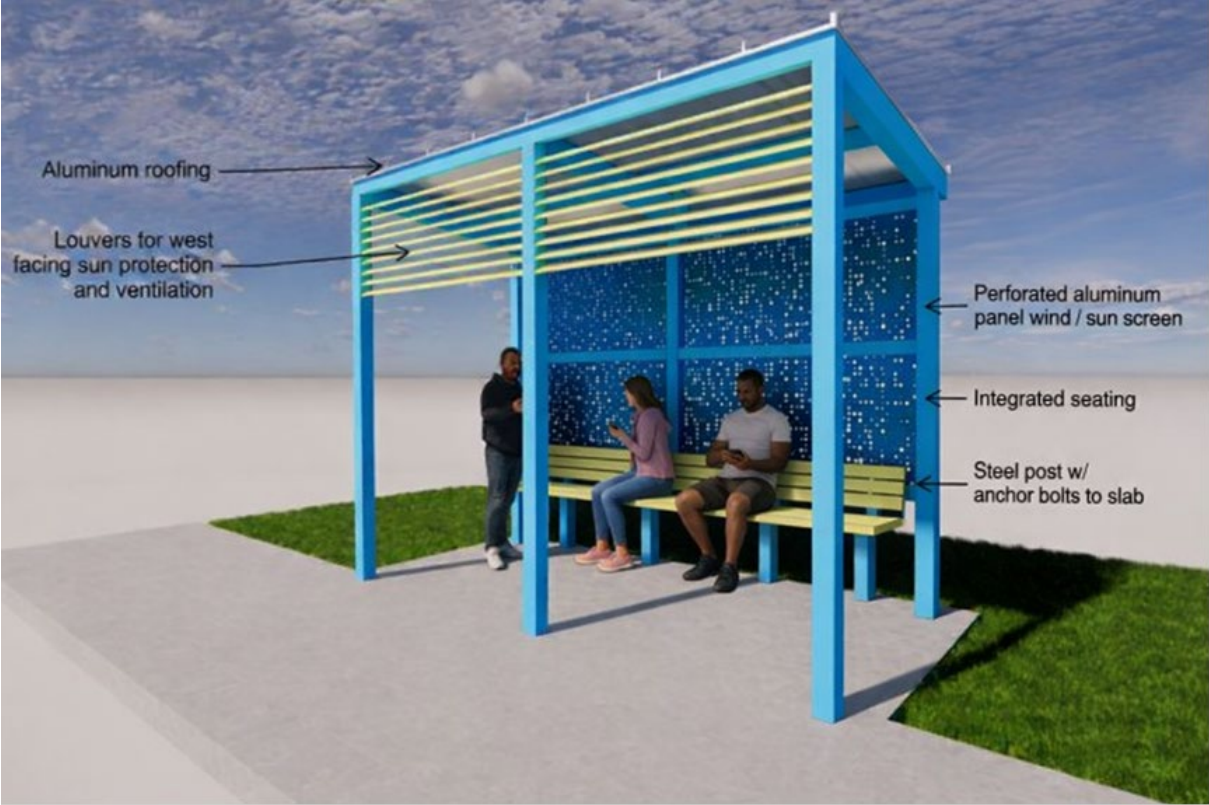
FIGURE 4-4. BUS SHELTER DESIGN USES PERFORATED PANELS AND LOUVERS TO MAXIMIZE SUN SCREENING AND ALLOW VENTILATION
