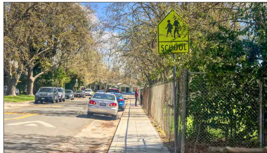
Existing school warning assembly on 7th Avenue is obstructed by overgrown landscaping.
