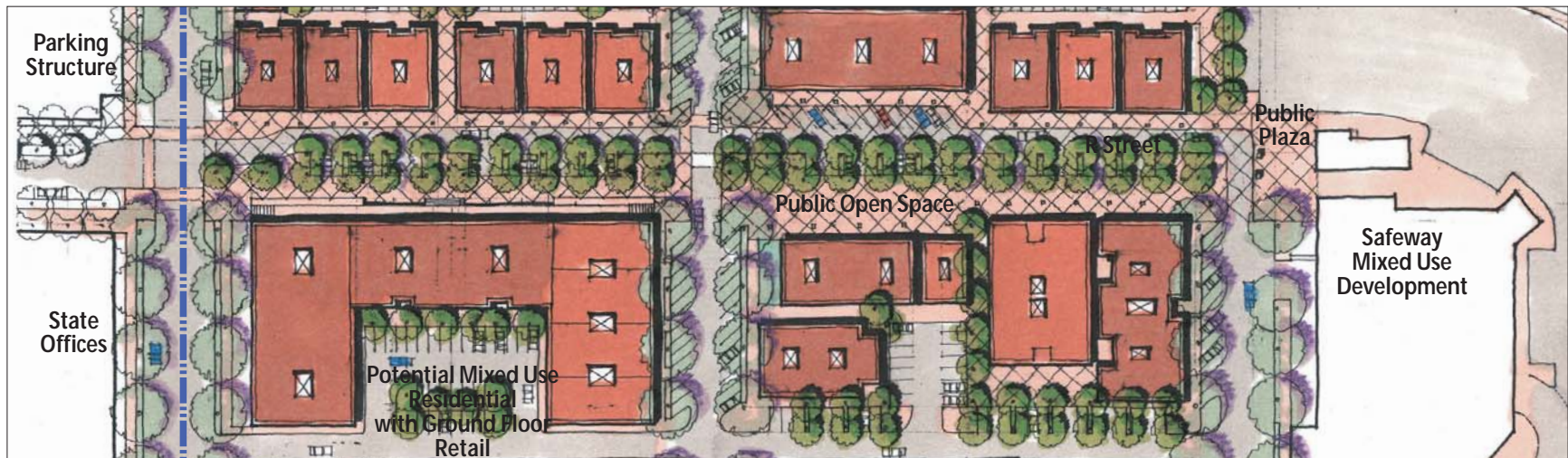
The Market Green is a two-block long multi-use public open space within the existing underused R Street right-of-way that connects to the recently completed R Street Market
