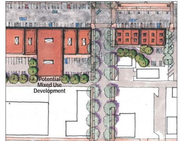
Mid-block alleys provide vehicular access to buildings and parking lots.
