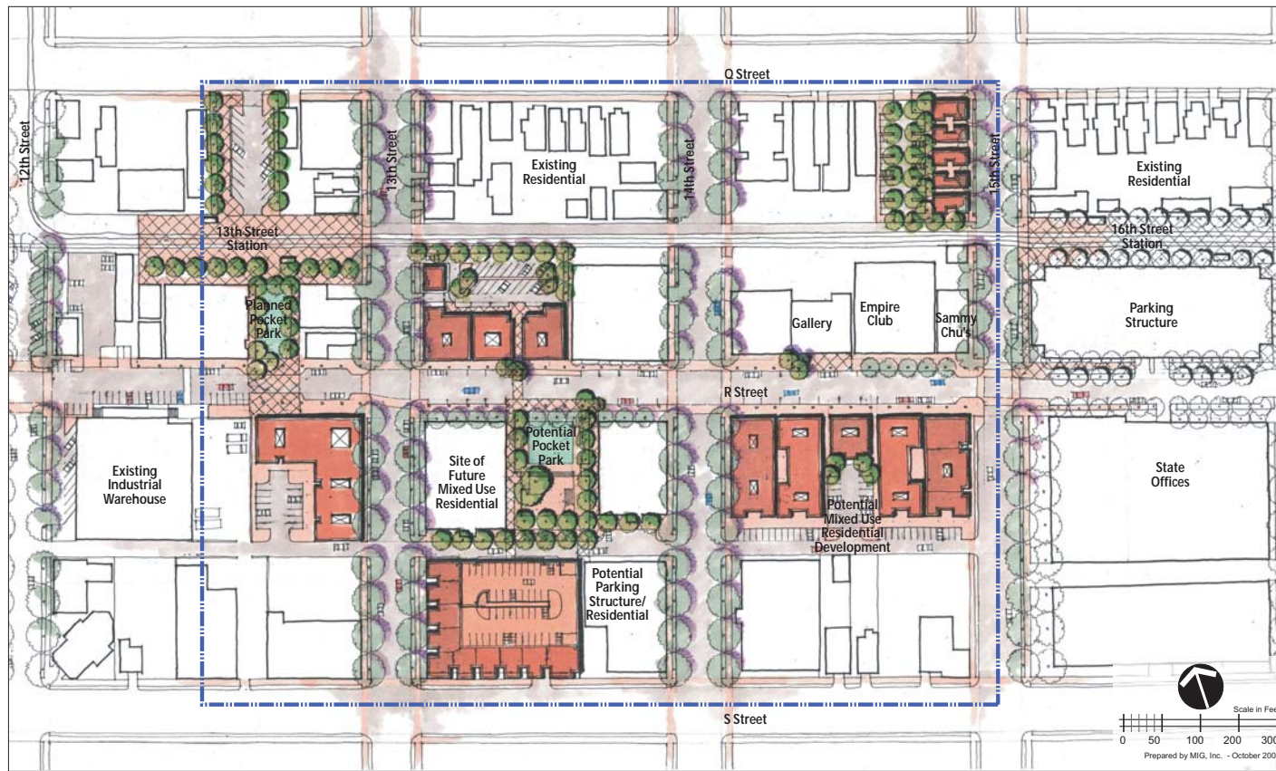
Figure 4.15 is a conceptual plan sketch. After this sketch was completed it was determined the street right-of-way is not sufficient for 90 degree parking; however, angled parking will be explored in the detailed design.
