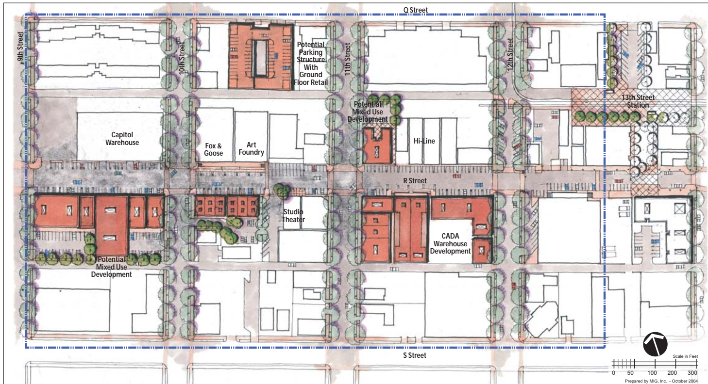
Figure 4.11 is a conceptual plan sketch. After this sketch was completed it was determined the street right-of-way is not sufficient for 90 degree parking; however, angled parking will be explored in the detailed design.
