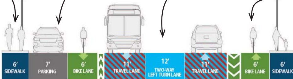
ROAD DIET WITH BUFFERED BIKE LANES WITH CENTER TURN LANE 36th Street to 38th Street
