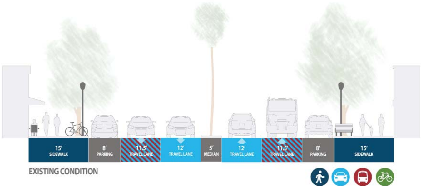
FIGURE 3: EXISTING CROSS SECTION
