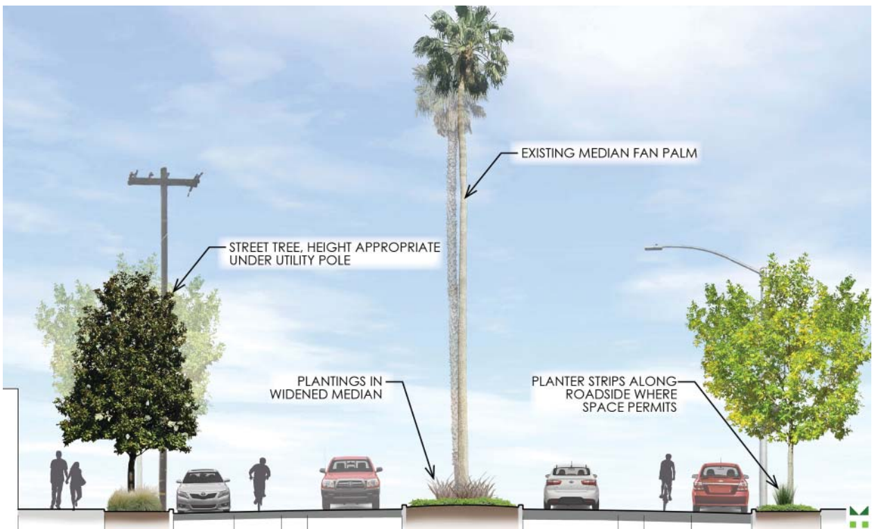
FIGURE 16: PREFERRED CROSS SECTION RENDERING
