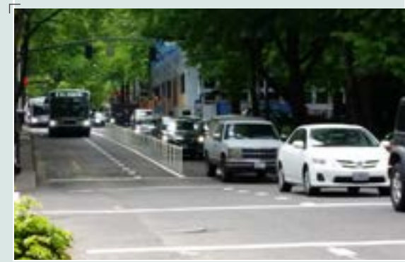
Bus-bike lane in Portland, OR lets the bus bypass traffic
