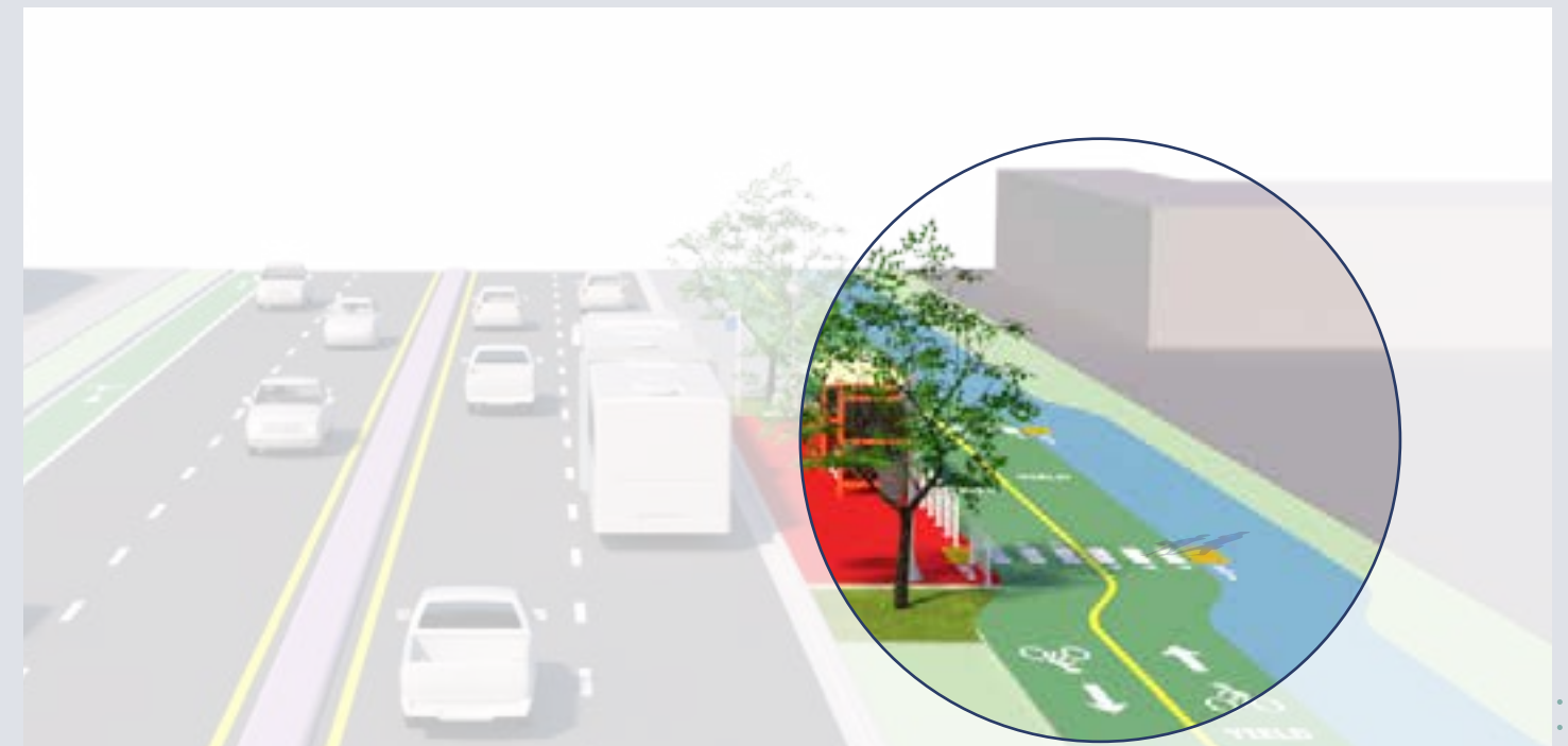
Two-way cycle track and sidewalk on the east side of the street can be achieved in collaboration with UC Davis as part of the Aggie Square development
