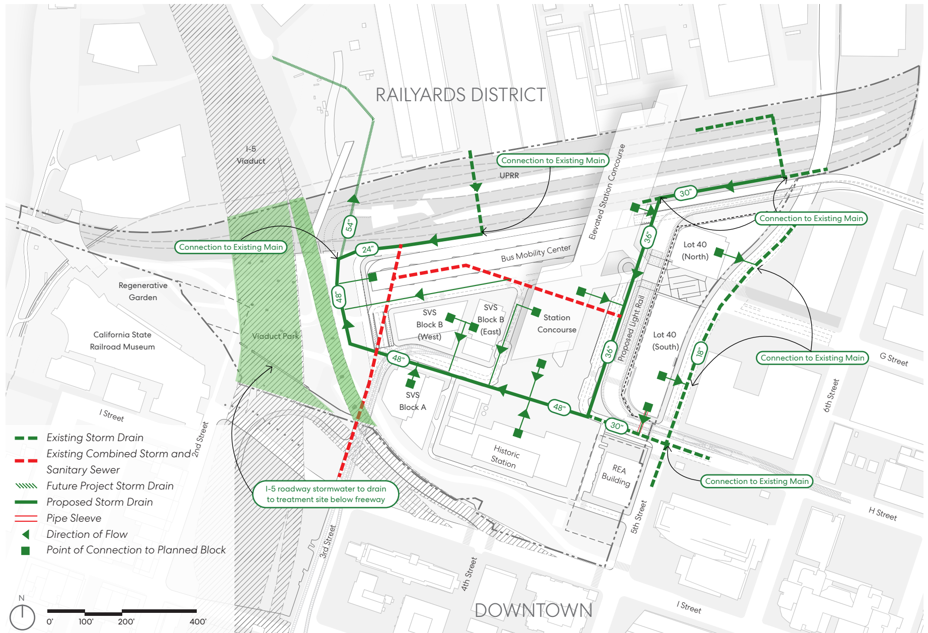
Figure 7.9 Utilities - Storm Drainage
