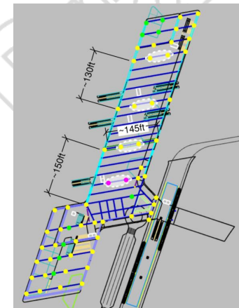
Figure 5 Concourse column grid. Yellow - columns from grade to Concourse Roof, green - from concourse floor, pink - from concourse floor to roof. Columns enclosed in a dotted white oval are moment frame columns to resist lateral load transverse to the bridge truss.
