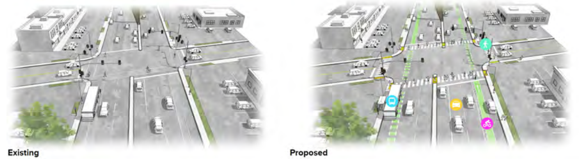
South Segment - From Harian Way to Oregon Drive Proposed Concept 2: Buffered Bike Lane
