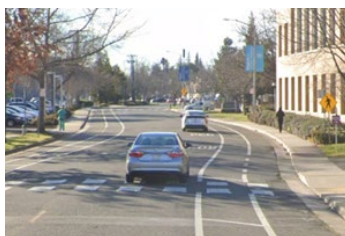
Midblock Crossings facilitate crossing to places people want to cross where no stop signs or traffic signals regulate the crossing.
