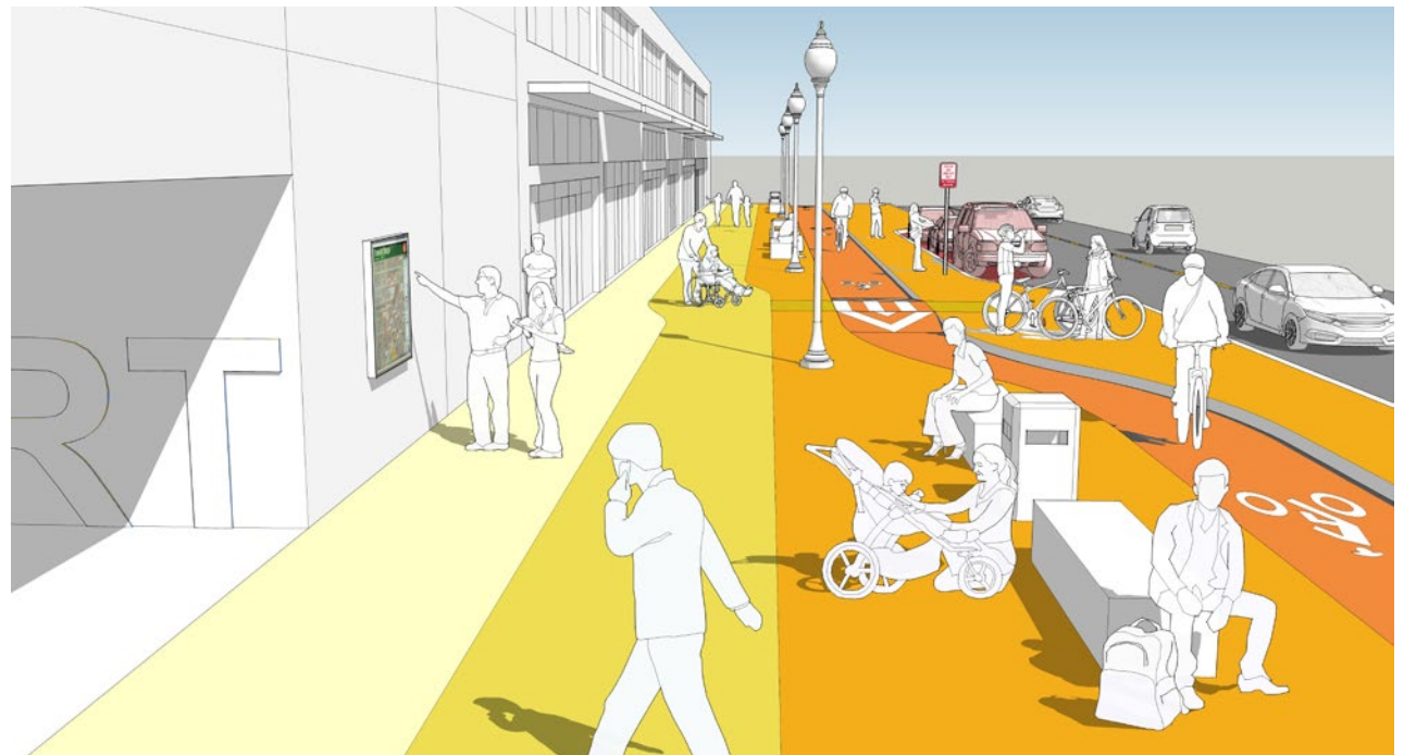
Figure 3.3.9: 3D View of Pick-Up and Drop-off Configuration Image credit: Robin Chiang & Company and Nelson\Nygaard
