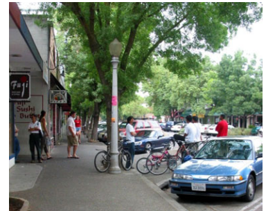
Angled parking provides a wide buffer between the sidewalk and adjacent vehicle lanes.
