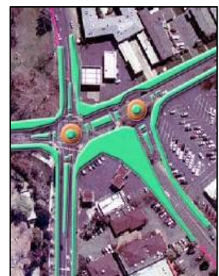
“Barbell” roundabouts would reduce pedestrian crossing distances
