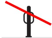
This style typically does not appropriately support a bike's frame at two separate locations.
