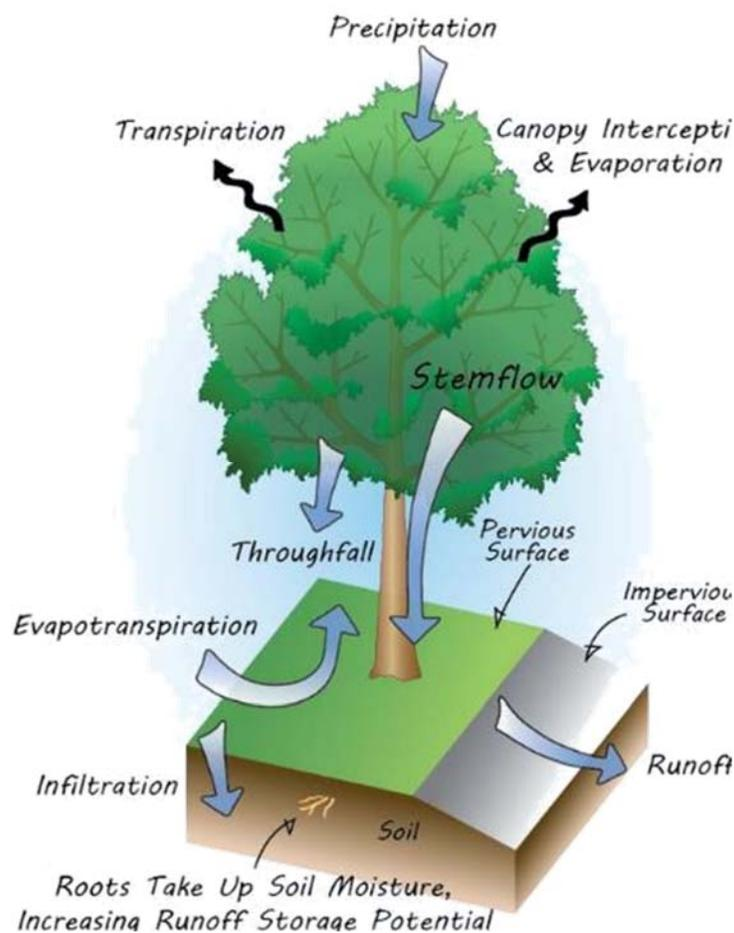
**Figure 5: Stormwater Runoff Diagram**
