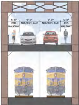
Proposed Bridge Cross Section
