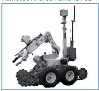
A remote-controlled, uncrewed machine that operates on the ground. A heavy-duty robot, with stair climbing ability and an arm capable of lifting 65 pounds.
