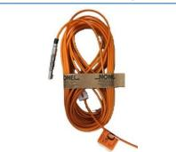
Sensitive primary explosive device used to initiate an explosive charge with zero delay.
