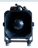
A device with a high-intensity, directional acoustical array for long-range communication.
