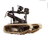
A remote-controlled, uncrewed machine that operates on the ground. A light-duty robot, equipped with an arm.
