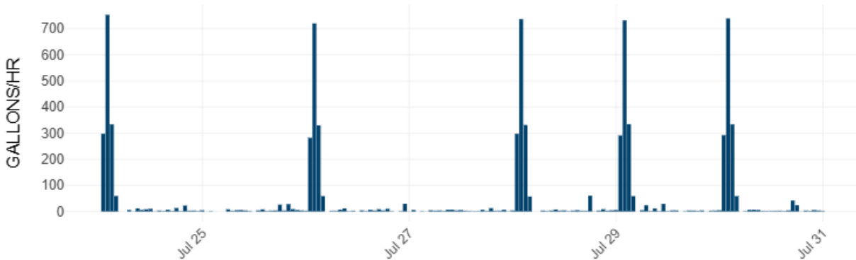
Figure 5-5. Service Address with 6 Days of Irrigation Using Up to ~500 gallons/hour
