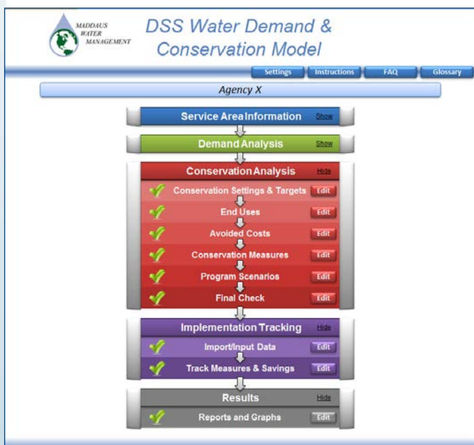
Figure AP-1: Schematic of DSS Model as applied to an urban water agency or regional area for water conservation
