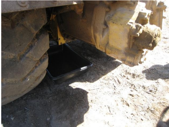
Appropriate – Drip pan provided when vehicle not in use.
