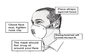
For a respirator that relies on a tight seal to the face, check how well it seals to the face by following the manufacturer's instructions for user seal checks. Adjust the respirator if air leaks between the seal and the face. The more air leaks under the seal, the less protection the user receives.
