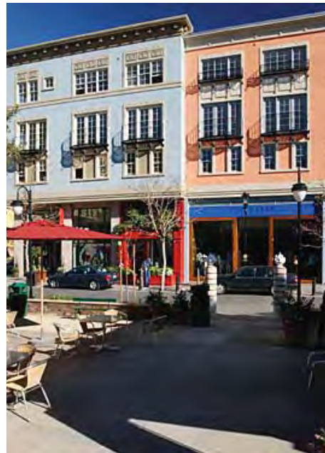
Windows, entries, and doors should occupy most of the wall surface on the ground floor of buildings fronting onto a plaza.
