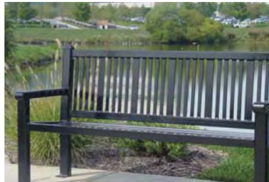
Stand alone street furniture should be constructed of cast metal with a powdercoated finish in colors and styles that complement the style of the commercial architecture.
