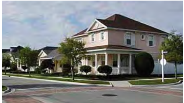
Housing facades on corner lots should provide architectural features that emphasize street presence on both streets.
