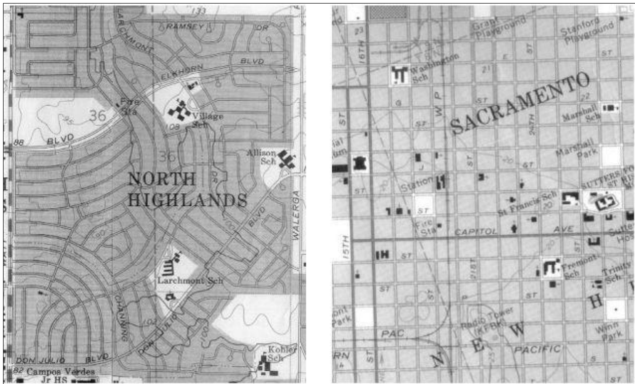
Figure 43. Comparisons of postwar and prewar street layouts: At left is a portion of the North Highlands tract near Sacramento, built in the early 1950s. It exhibits the characteristic street layout of the period, including curved streets, long blocks, and a limited number of through streets. More than two-thirds of the intersections shown are three-way intersections. At the same scale at right is a portion of central Sacramento, platted in the 19 th century. This older area has shorter blocks and about 100 more intersections, nearly all of which a four-way intersections. Blocks are narrower in North Highlands because there are no alleys. Source: USGS “Rio Linda,” “Citrus Heights,” and “Sacramento East” quads, 1967.
