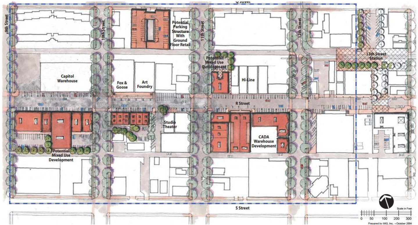
Figure 6-43. is a conceptual plan sketch. After this sketch was completed it was determined the street right-of-way is not sufficient for 90 degree parking; however, angled parking will be explored in the detailed design.
