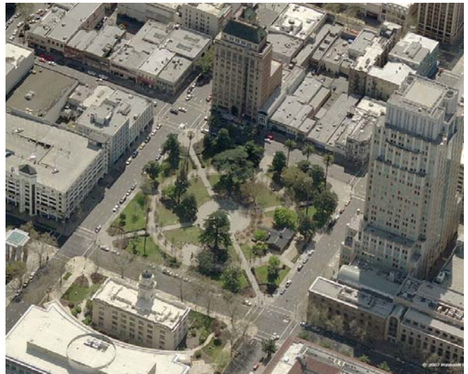
The streets surrounding Cesar Chavez Plaza are built up with consistent street walls and zero setbacks that are appropriate for this downtown location.
