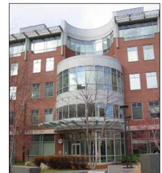
Figures 7 & 8. Different materials and colors should be separated with a change in plane.
