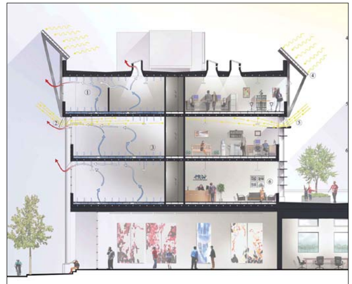
Figure 5. Cross section of an office building showing integrated ventilation and daylighting strategies.
