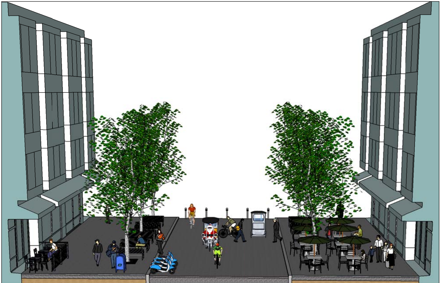
Figure 3.18. This cross section perspective view shows the dominate pedestrian streetscape with provision for delineated vehicular way separated with a four inch high curb for cyclists, peddle cabs, and other light vehicles that can mix with crossing pedestian movements. These design elements will contribute to a unique and identifiable urban place which can support community venues and local festivals.
