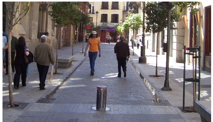
As a component of residential alleys, retractable bollards can limit vehicular access to alleys with electronic coding
