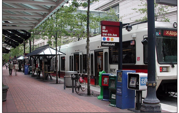
Figure 3.46. Light rail curb-side stations in downtown Portland, Oregon provide passenger amenities with generous sidewalk widths for passenger waiting and pedestrian throughway. Note projecting awnings from buildings that provide additional shelter for passengers.
