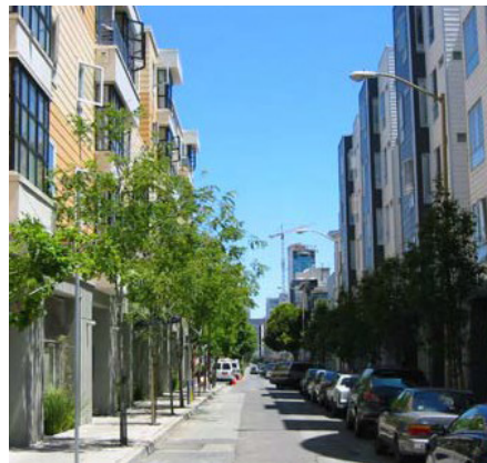
Figure 4-186. Redevelopment along both sides of Natoma Street, one of the narrow alley-like streets that subdivides the giant blocks South-of-Market in San Francisco. The right of way is just 35', but still wide enough for sidewalks, one-way traffic and on-street parking.
