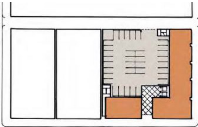
Figure 4-241. One-Level Podium Parking (Corner Parcel)
