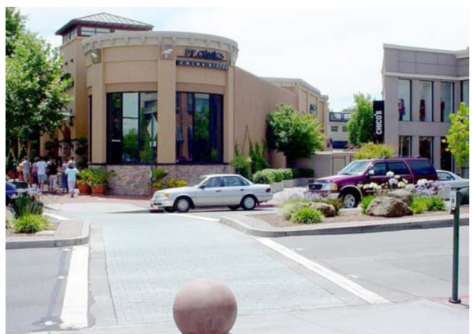
Figure 3-30. Special paving treatments and pedestrian-activated crossing lights alert drivers to the presence of pedestrians.
