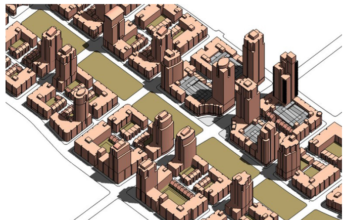
Figure 2-21: This hypothetical urban design study follows the tower separation guidelines. Towers are always at least 80' apart, and there are never more than the permitted four towers per block.
