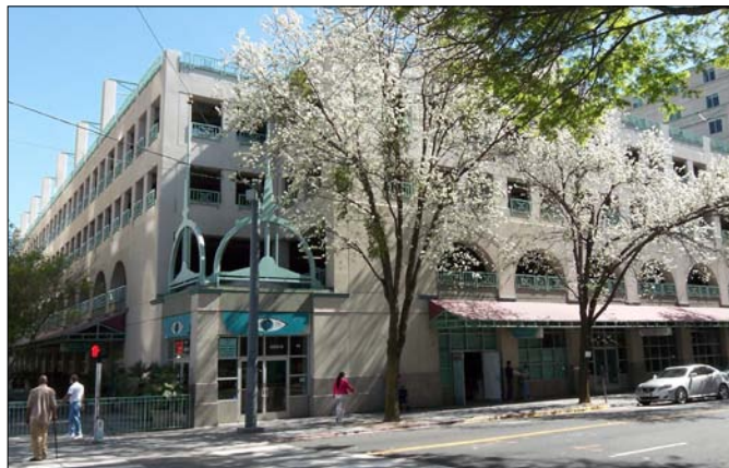
Figure 5. The Hyatt parking garage, where the facades are designed in manner consistent with the overall project. The street-facing facade is articulated with a rhythm of archways ending in a notched entry corner.
