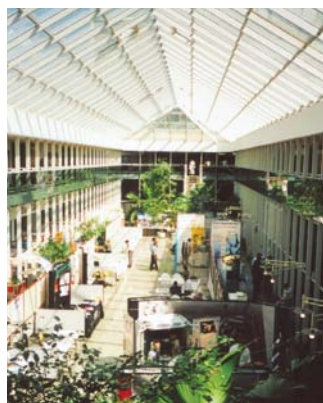
Figures 3 and 4. Internal sky-lit atria, allowing daylight light to penetrate to a maximum amount of internal space, at all floors
