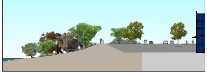
Figure 3.30. Berming behind levee at Township 9, allows parking garages built on existing grade with new fill graded to surround parking with elevated ground plane.
