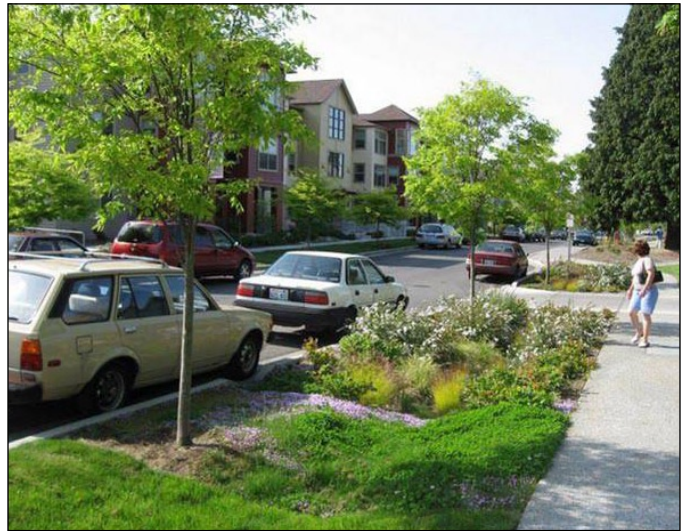
Figure 3.44. Bioswales provide valuable function to filter runoff and mitigate surges of runoff in peak rain events. They also provide aesthetic enhancement to the public way.
