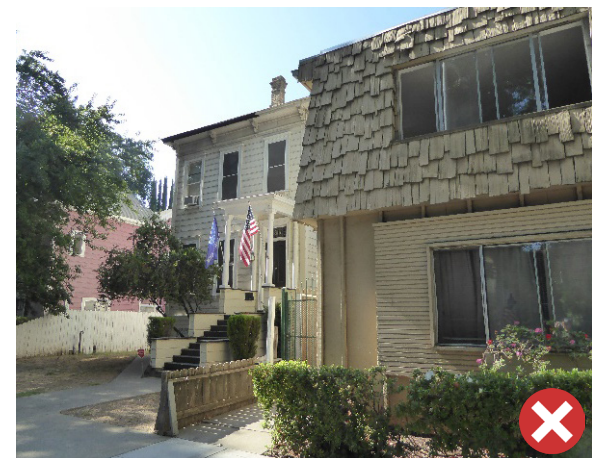
Figure 198. The apartment building on the right does not align with the setback of the historic house on the left.
