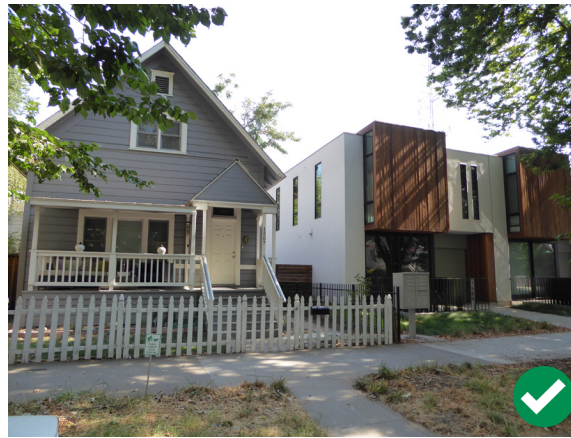
Figure 33. These new apartment buildings match the setback, scale, and street-facing orientation of adjacent contributing buildings.
