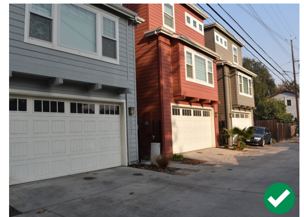
Figure 65. Windows and entries facing the alley are recommended. The taller massing of these buildings has also been broken down into smaller components to reflect the scale of buildings in the surrounding neighborhood.
