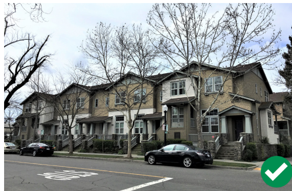
Figure 34. The larger massing of this multi-family residential building has been broken down into smaller modules that relate to the surrounding neighborhood.
