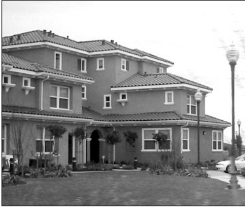
Multiple roof lines can reduce the appearance of mass in large multi-family structures.
