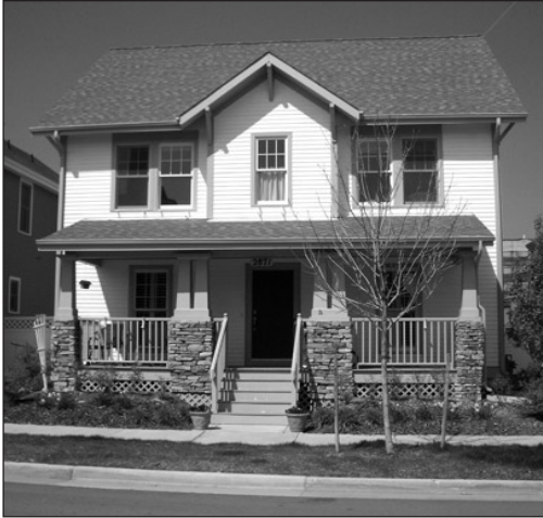
Architectural details and articulated facades can help to minimize the appearance of two-story infill homes.
