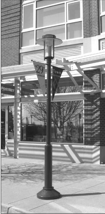
Pedestrian pole lighting with a solid top eliminates light spillover and glare.
