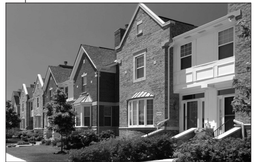
Bay windows and architectural detailing help to articulate the facade and reduce the appearance of mass in these two-story duplex units.
