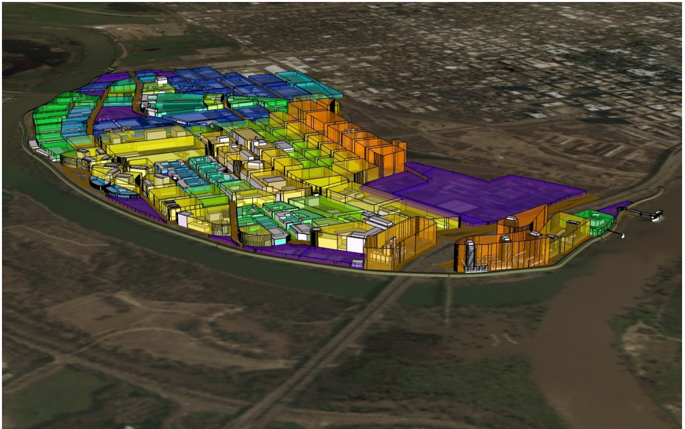
Figure 2.5. Allowable height diagram of RDSP blocks illustrates 250 ft height envelope (orange) at confluence of Sacramento and American Rivers, and lower height envelopes along American River Parkway.
