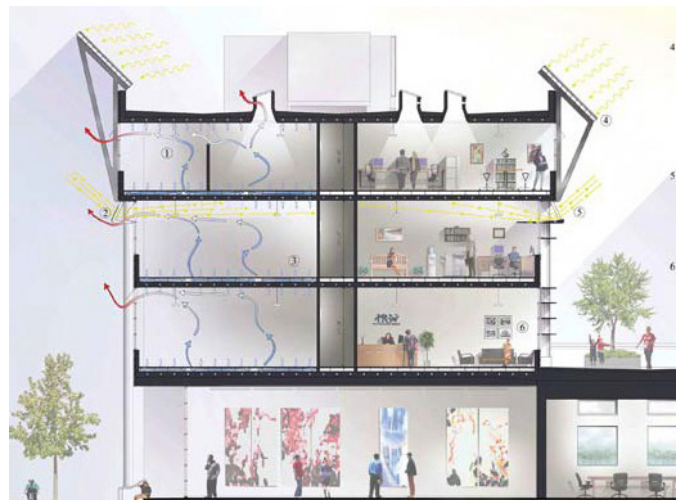
Figure 4-204. Cross section of an office building showing integrated ventilation and daylighting strategies
