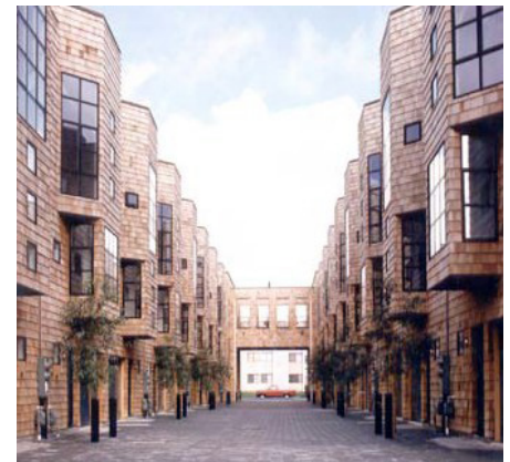
Figure 4-187. Fulton Grove, San Francisco, is an example of a residential alley with dwellings fronting the right-of-way. Unit pavers, front doors and no curbs make this a pedestrian friendly environment.
