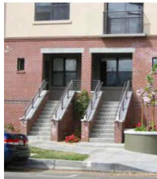
Figure 4-143. Entrances to individual units should orient to the street & be characterized by stoops, porches etc.
