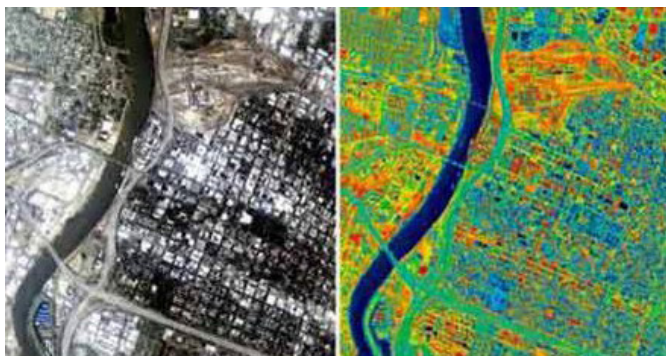
Figure 4-193. NASA fly-over photograph of Sacramento, July 1998 (left), Thermally sensed image of Sacramento (right).
