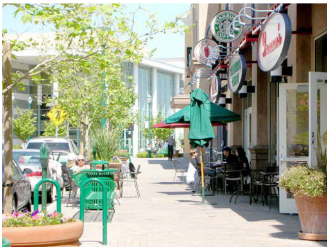
Figure 3-42. Three functional zones of public sidewalks: Public Amenity Zone, Pedestrian Zone, and Frontage Zone.
