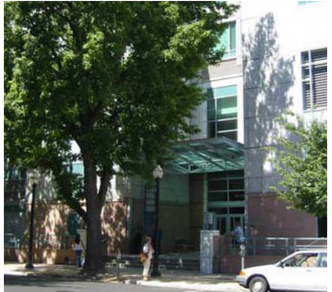
Figure 3-87. The east entry of the cal/EPA Headquarters building was setback around the canopy of an existing street tree. As a result, the tree provides strategic shade to a highly trafficked user route
