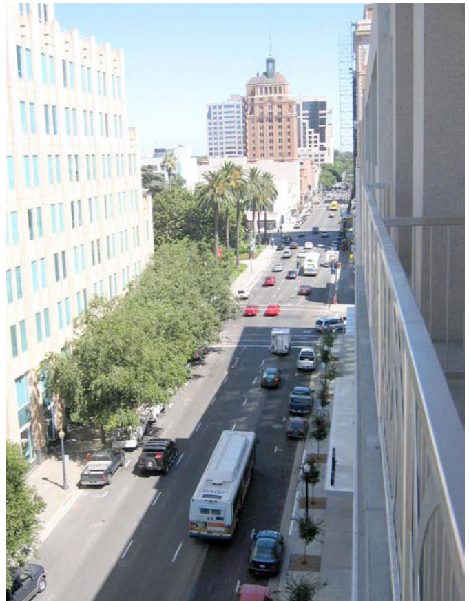
Figure 3-3. The travelway generally occupies 60 to 65% of the public right-of-way.
