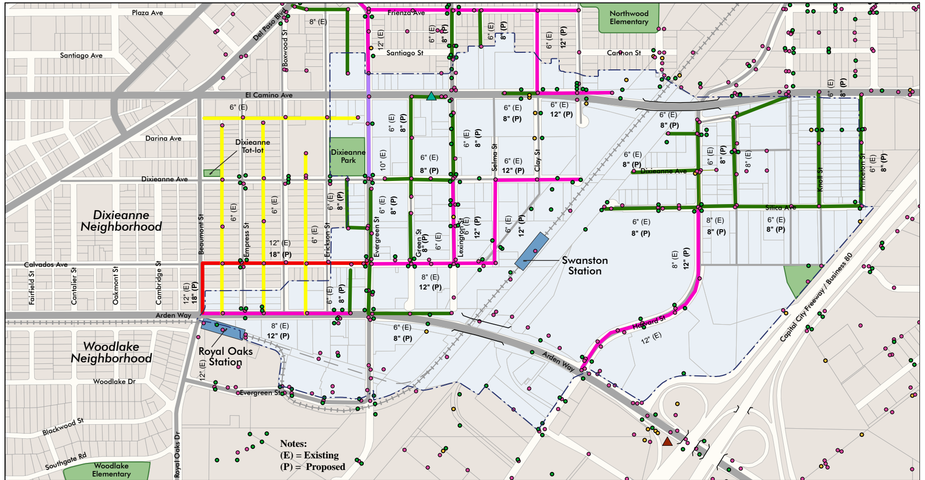
FIGURE 3.4 RECOMMENDED SANITARY SEWER IMPROVEMENTS
