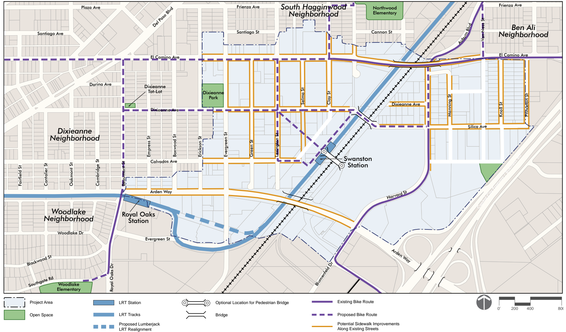
FIGURE 2.5 RECOMMENDED PEDESTRIAN AND BICYCLE SYSTEM IMPROVEMENTS
