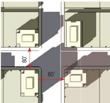
Figure 2-20: Towers should be spaced at least 80' apart from each other, the equivalence of a street width, and vary considerably in height from those closest to it.
