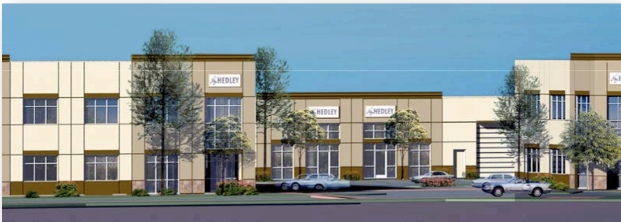
Image 2.2: Use of varying building heights, massing, and setbacks are utilized to break up the building's massing and minimize bulk
