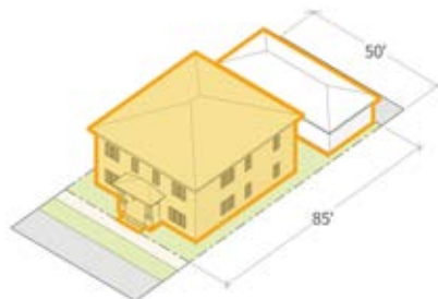
1 parking sp/unit (alley access) Fourplex needs a deeper lot Density achieved: 41 du/ac
