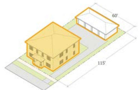
1 parking sp/unit (front driveway access) Fourplex needs a deeper, wider lot Density achieved: 25 du/ac
