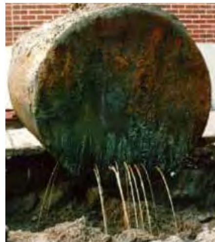
An example of a leaking underground storage tank (not in Sacramento)
