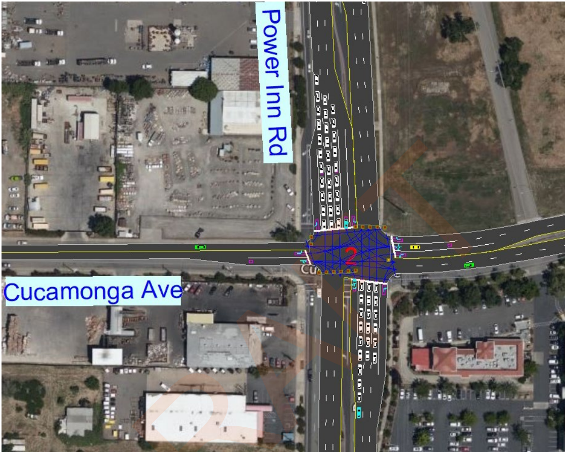
Illustration 2: Simtraffic screenshot showing of northbound left-turn by through traffic during pre-event peak hour.
