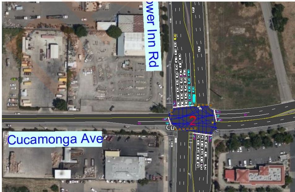
Illustration 1: Simtraffic screenshot showing blockage of southbound right-turn by through traffic during pre-event peak hour.
