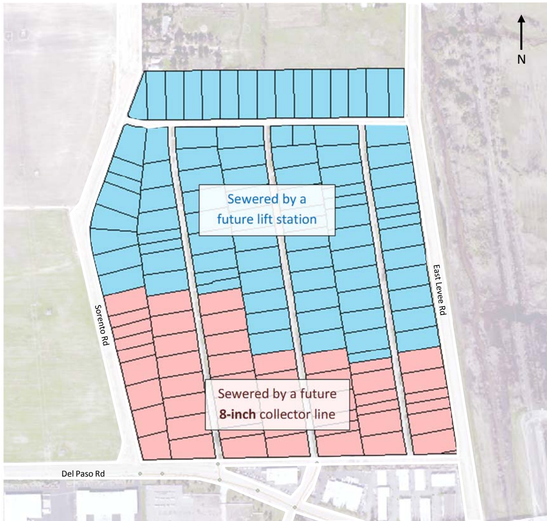
Figure 2. Plan view map of how the Valley View Estates will be sewered based on the Natomas Panhandle Sewer Study
