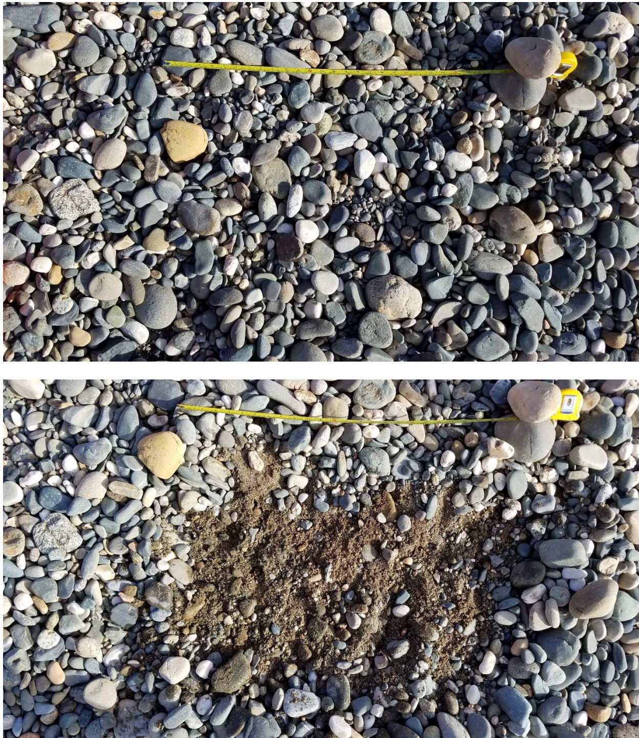
Figure 2.5. Surface (top) and sub-surface (bottom) bed material at River Bend (samples 9a and 9b).
