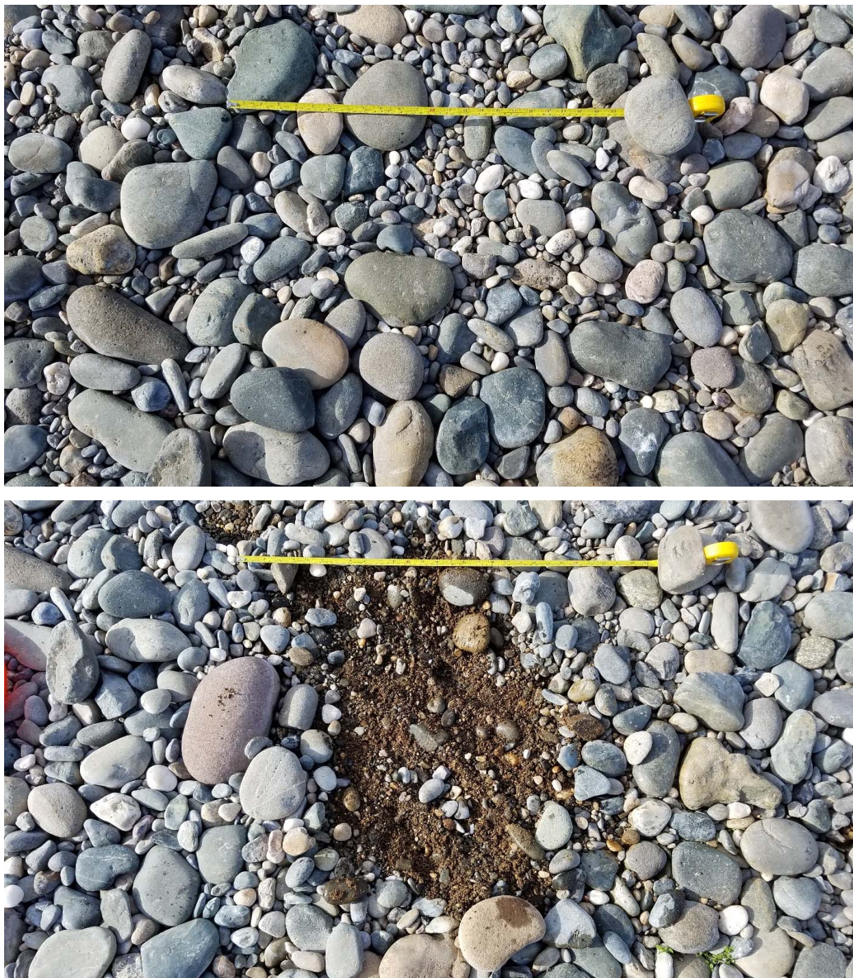
Figure 2.4. Surface (top) and sub-surface (bottom) bed material at Lower Sunrise (samples 6a and 6b).
