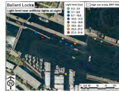
FIGURE 45. Light level readings (lx) in selected areas of the Ballard Locks study site. Selected areas used more intensively by tagged Chinook salmon are outlined in black. See Figure 38 for distribution of tagged Chinook salmon usage intensity. Ambient light level was generally 0.0 lx, although in some areas was as high as 0.2 lx.
