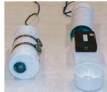
Figure 2. Photograph showing the Sky Quality Meter installed in its protective housing (SQM-LU left), along with an expanded view (SQM-LE right). The housing at left is shown with the two included hose clamps that allow easy attachment to a stake or pole. The USB version (left) requires only one cable, but at the cost of shorter cable runs and the internal heating provided by the Ethernet version (right). doi:10.1371/journal.pone.0017307.g002
