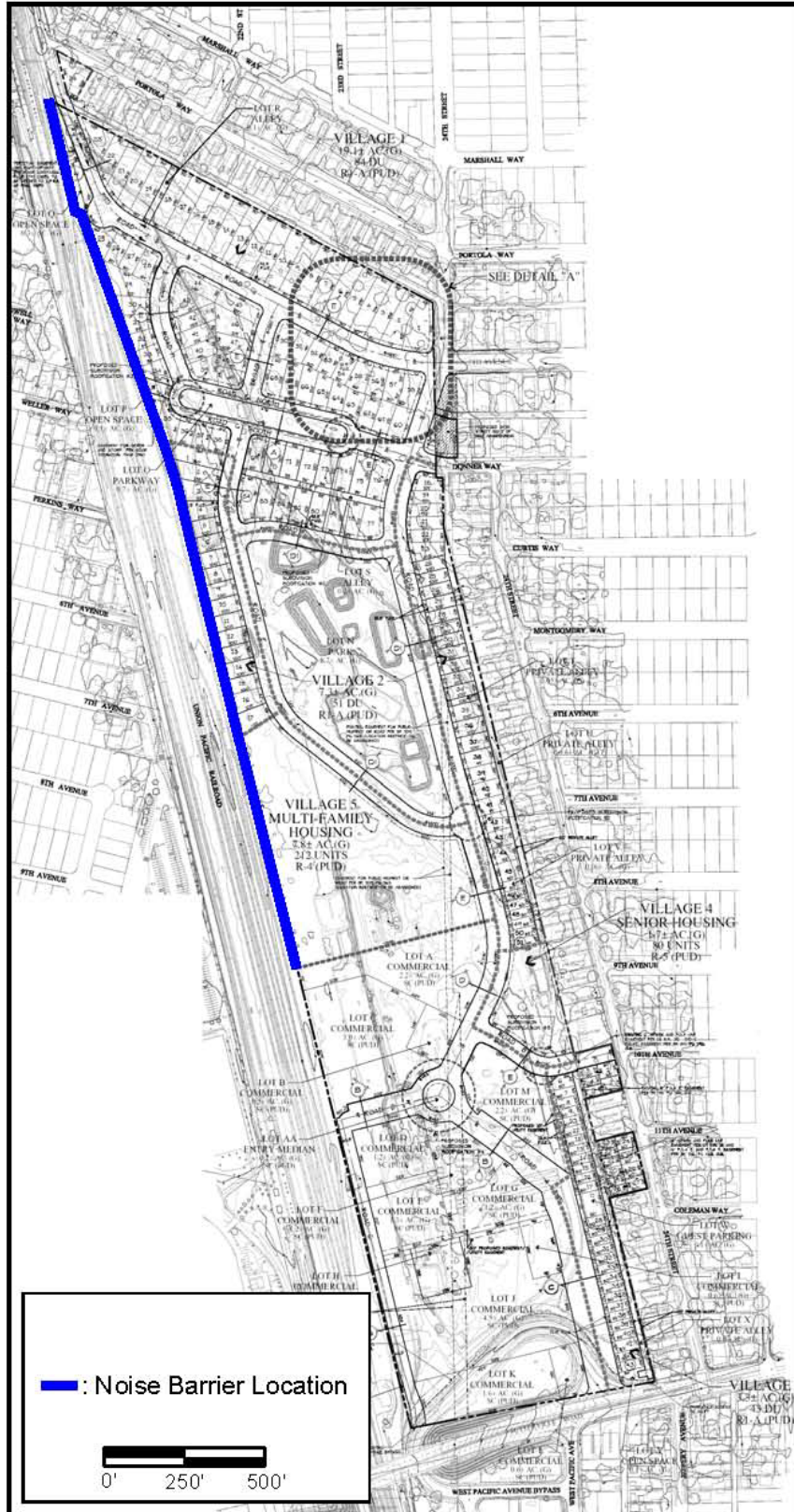
Figure 5.4-2 Noise Barrier Locations
